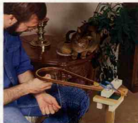
The author built this stand to clamp his work when he's hanging nets. It holds the net frame, so Carson's hands are free to attach the net. Using a length of 50#-test monofilament, which measures twice the length of the frame's perimeter (minus the handle), Carson secures the net loops within the perimeter groove.
